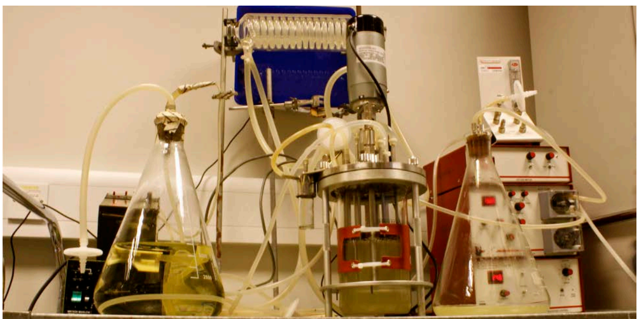
Illustration 19: Chemostat set-up, three-tier system with feed (left), fermenter (centre), and deposit (left). Photo: Howard Boland.
