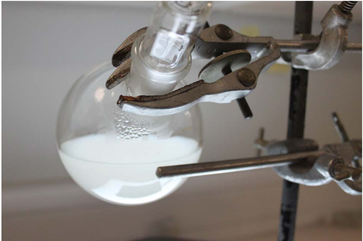
Illustration 46: Banana Bacteria final set-up with culture in Florence Flask (minimal media, knockout strain transformed with plasmid construct). Photo: Howard Boland.
