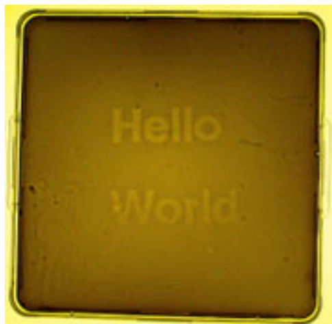
Illustration 50: Example of light sensor (also called bio-photolithography) in action (Levskaya et al., 2005). Permission to reproduce this image has been kindly granted by Anselm Levskaya.
