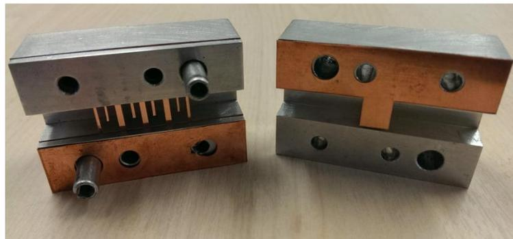
**Figure 4.5-20: Photograph of the fabricated inserts within the custom made split block waveguide housing for the 4<sup>th</sup> order E-plane Cross-coupled filter.**
