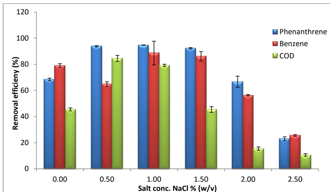
**Figure 4.3:** Effect of salt concentrations on COD removal and degradation efficiencies during MFC operation (at 30°C) using adapted anaerobic microbial consortia. Values are means of duplicate experiments  $\pm$  SD.
