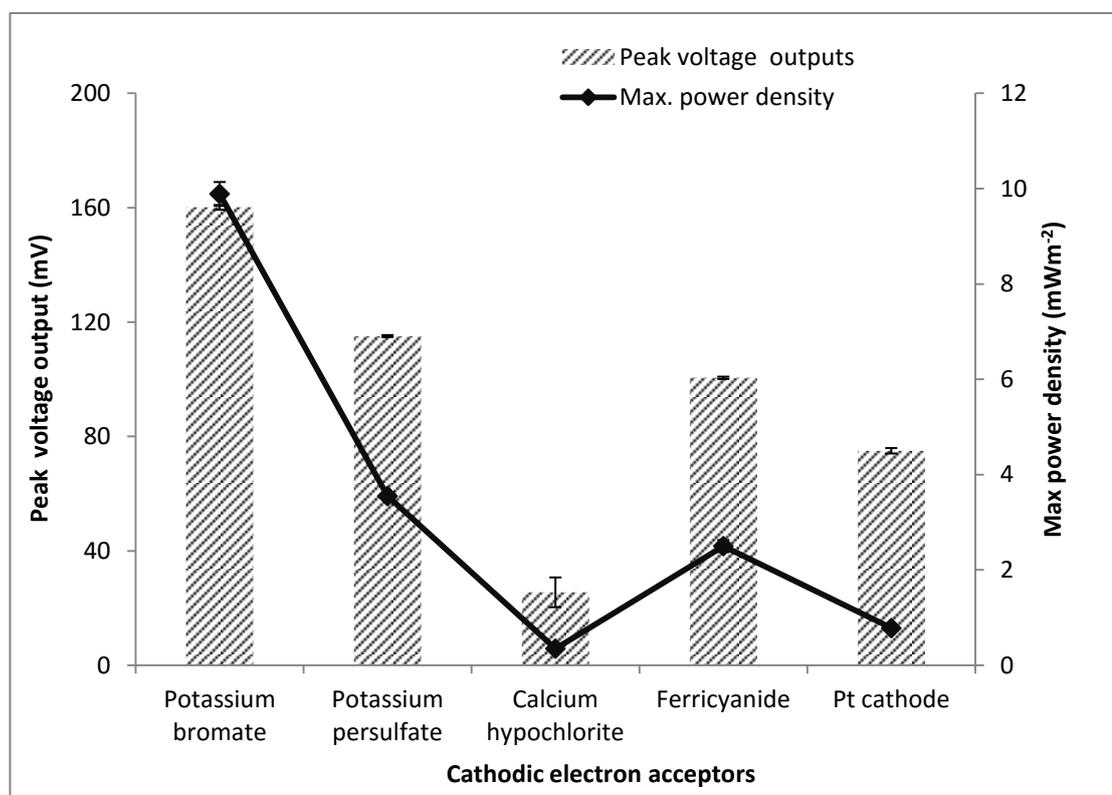
**Figure 4.7:** The electrochemical performance of the MFC using different electron acceptors at the cathode (Ext. resistance, R= 1 kΩ). Values are means of duplicate experiments ± SD.
