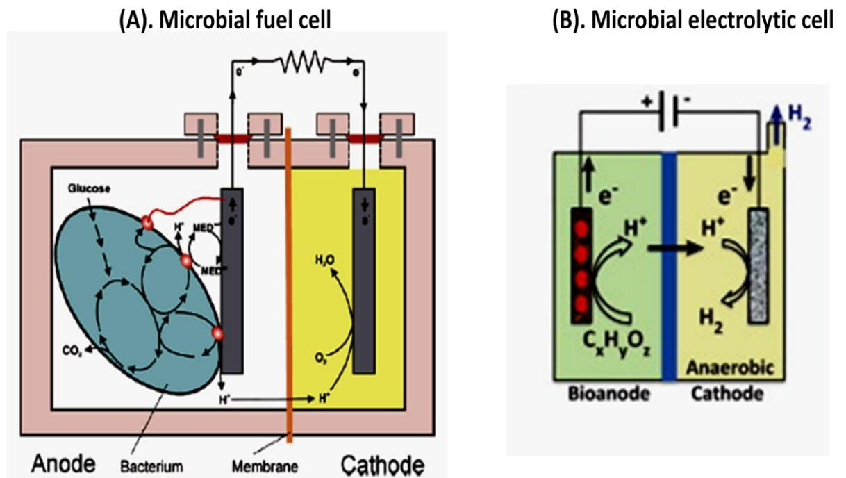
**Figure 1.14:** The operating principle of a microbial fuel cell (MFC) and microbial electrolysis cell (MEC) (images adapted from Han et al., 2013 and Logan et al., 2006)
