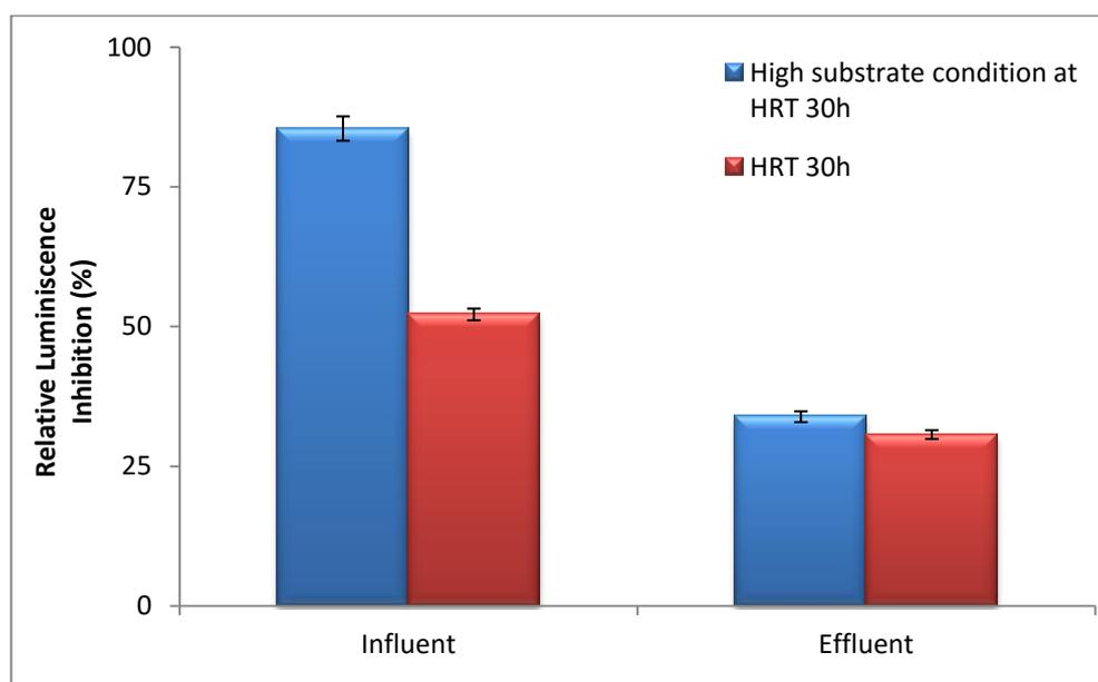
**Figure 5.9:** Toxicity levels of MFC effluents at HRT 30h and high substrate condition using adapted microbial consortia as inoculum source. Values are means of duplicate experiments  $\pm$  SD.
