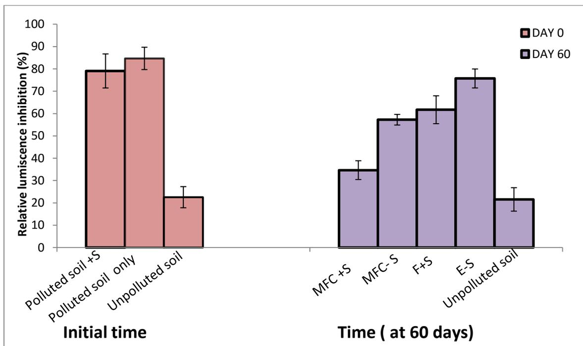
**Figure 6.9:** Toxicity levels in soil extractions of polluted soil with and without MFC treatment operated at 25-30°C over 60 days incubation period. The error bars represent 5% of deviation of the mean value for triplicate measurements. MFC-S and MFC+S are MFC only and MFC with surfactant (Tween 80, 250 mg L<sup>-1</sup>) amendment respectively. E-S and F+S mean controls without and with surfactant addition respectively.
