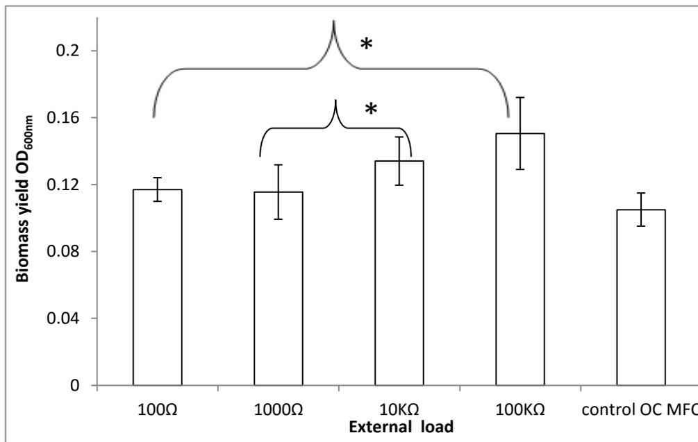
**Figure 4.11:** Total biomass yield measured at 600 nm under MFC operating with different external resistance and at open circuit (OC) MFC using adapted microbial consortia at incubation temperature of 30 $\pm$ 3 $^{\circ}$ C. Mean data from duplicate reactors with error bars ( $\pm$ SD). \* indicates data is statistically significant at  $p < 0.01$ .
