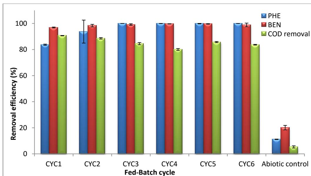
**Figure 4.1:** Percentage COD removal and degradation efficiencies of petroleum hydrocarbons mixture during MFC fed-batch operation using adapted microbial consortia. Values are means of duplicate experiments  $\pm$  SD. Data for abiotic control represent the average values over six cycles.
