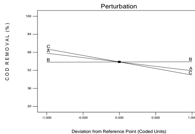
**Figure 4.16:** Perturbation plots indicating interaction effects of variables for each response factor; (A) TPH (Total petroleum hydrocarbons) (B) Power density and (C) COD removal. It should be noted that the chosen reference points for the factors; A (Salinity), B (External resistance), C (Redox mediator) are 1.0 % w/v NaCl, 50 kΩ and 30 μM Riboflavin respectively.
