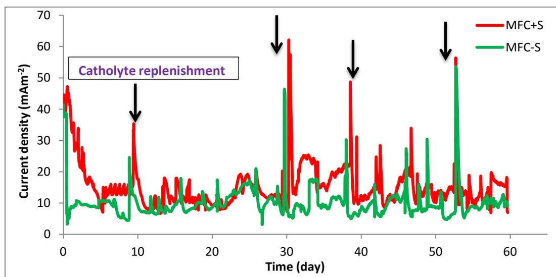
**Figure 6.6:** Current densities of MFC+S and MFC-S during the tubular MFC operations over 60 days incubation period ( $R_{\text{ext}} = 1000 \Omega$ ). Black arrows indicate the points for catholyte replenishment.
