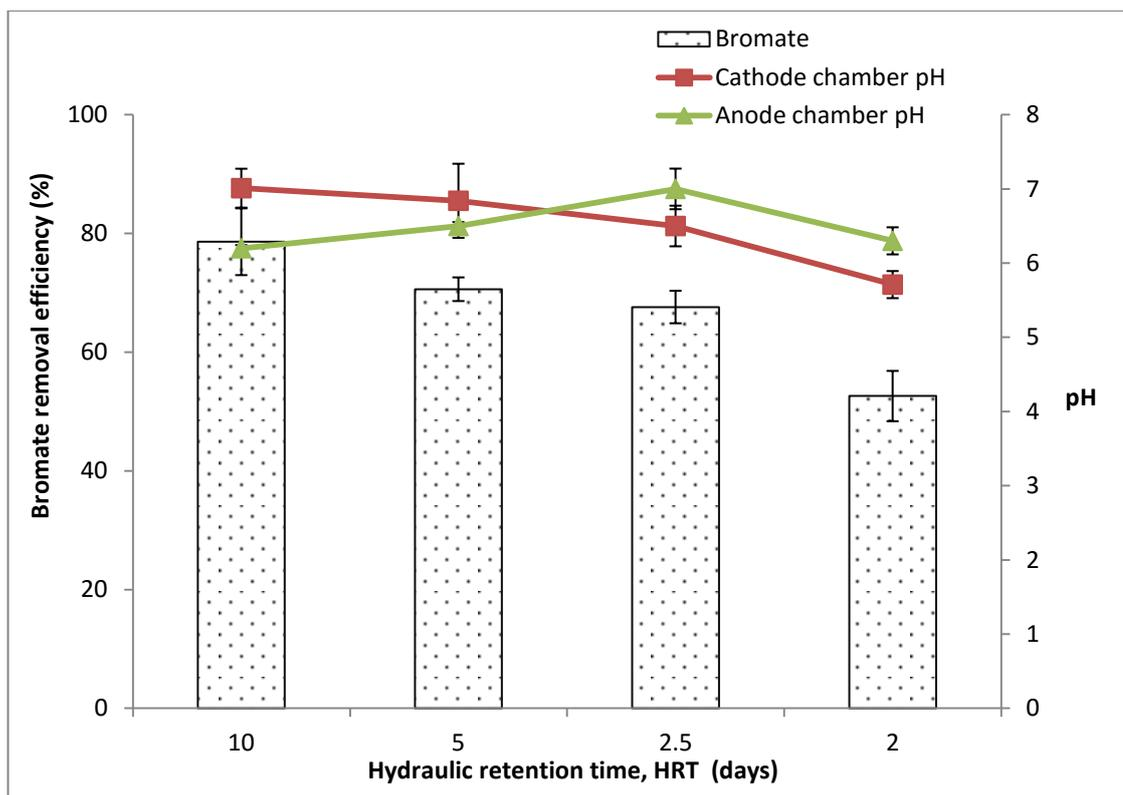
**Figure 5.4:** Bromate removal performances and changes in pH in the tubular MFC reactor over 110 days operation at ambient temperatures (10-25°C) using adapted microbial consortia. Error bars  $\pm$  SD are based on duplicate measurements.
