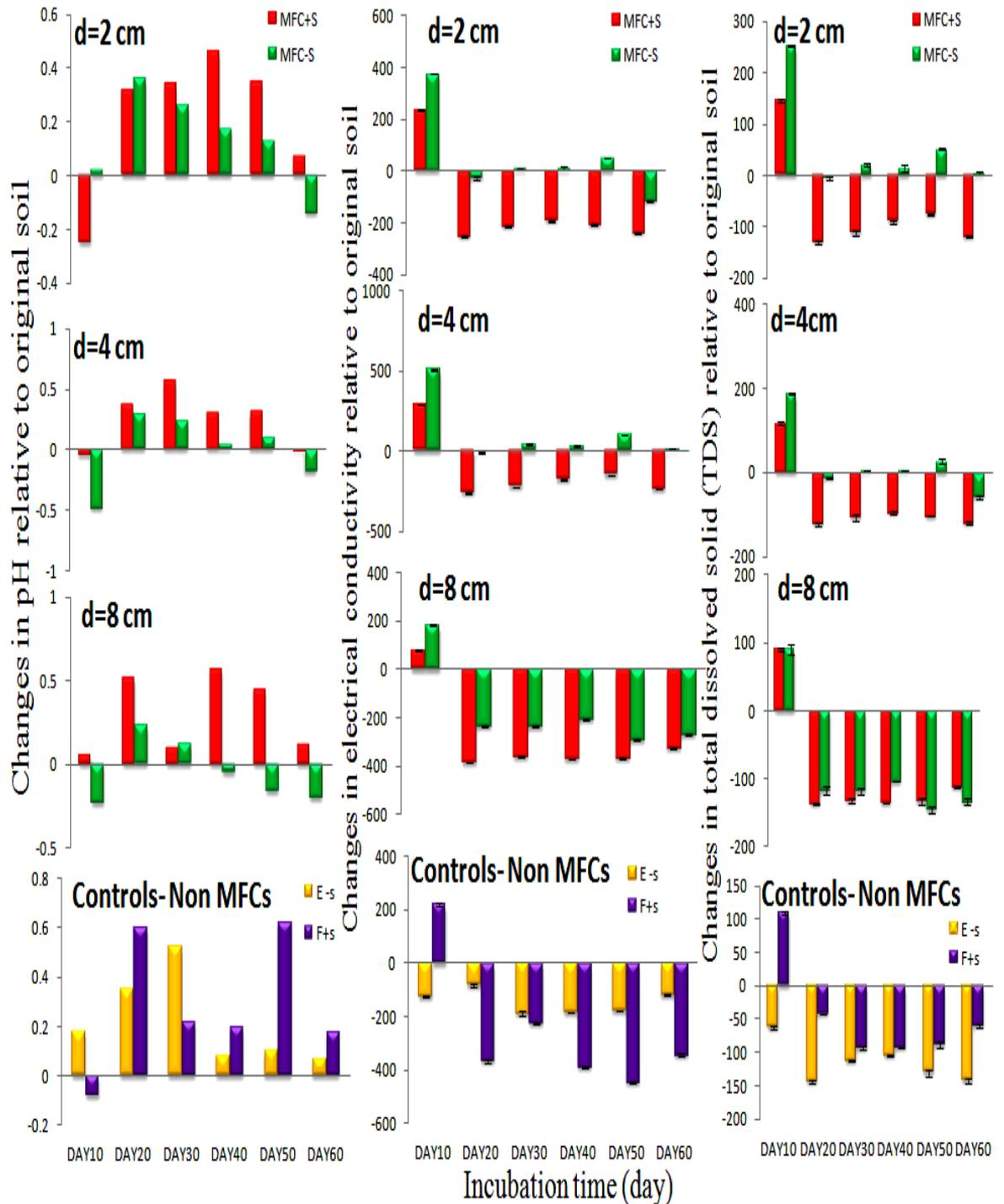
**Figure 6.8:** Changes in soil pH, TDS and electrical conductivity in MFC at different distance from anodes and control reactors over the tested period. The error bars  $\pm$ SD were based on averages measured in triplicates. E-S and F+S mean controls without and with surfactant addition respectively.
