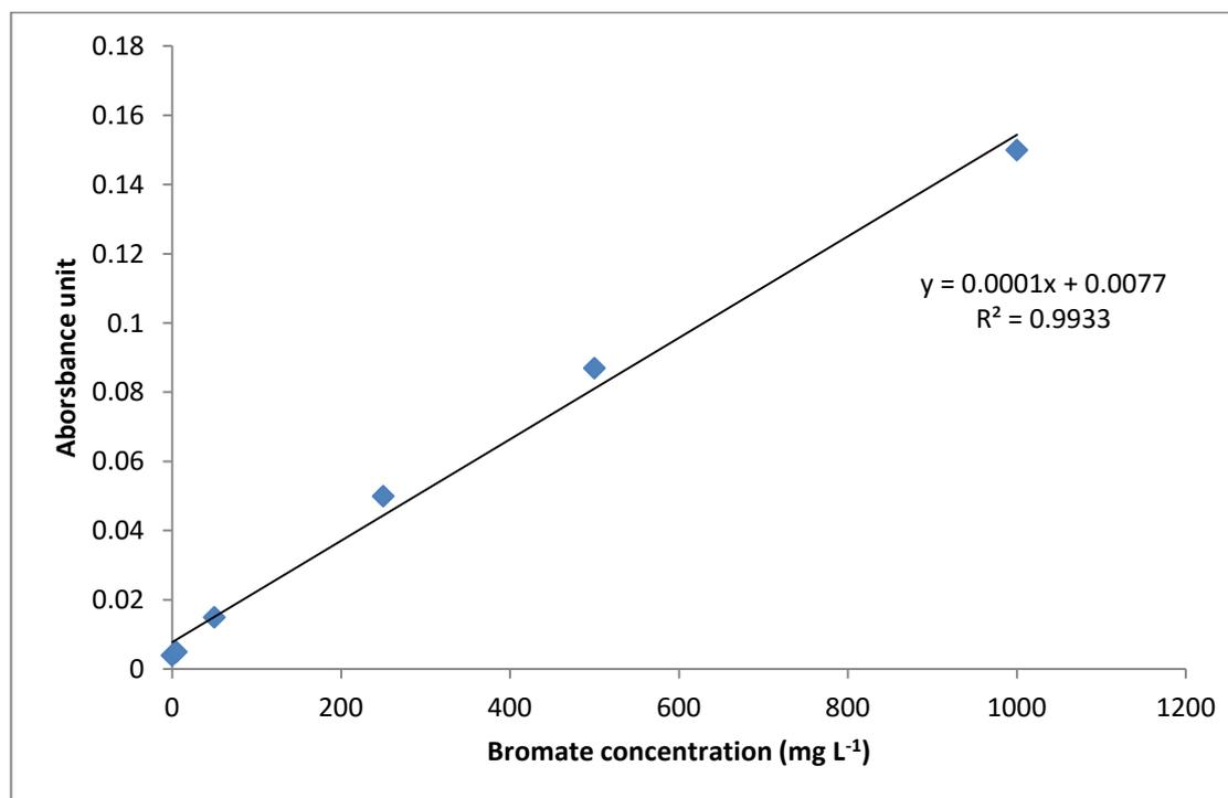
**Figure 9.1:** Calibration plot for bromate standard concentrations
