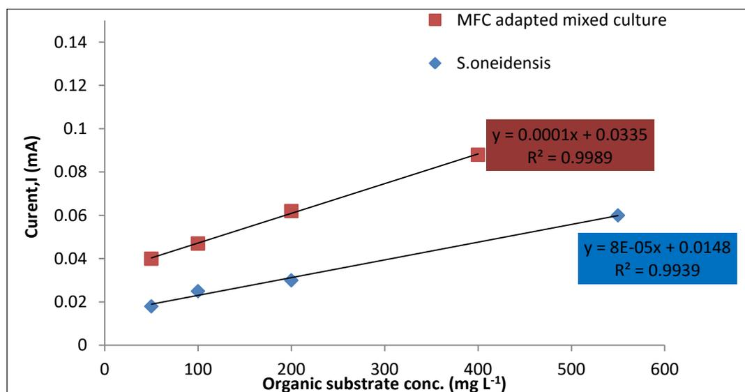
**Figure 3.13:** Relationship between organic substrate concentration and current generation from MFCs for different inocula (*S.oneidensis* and MFC-adapted mixed culture).
