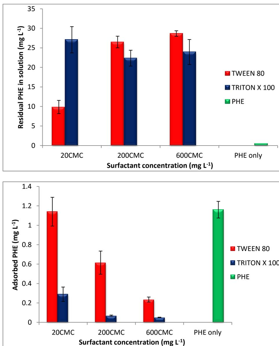
**Figure 4.8:** (A) Residual PHE (phenanthrene) present in the aqueous phase about 24 h after MFC operation began (B) Adsorbed PHE on the electrode after MFC operation for different concentrations of surfactants tested using adapted microbial consortia as inoculum source. Values are means of duplicate experiments  $\pm$  SD.
