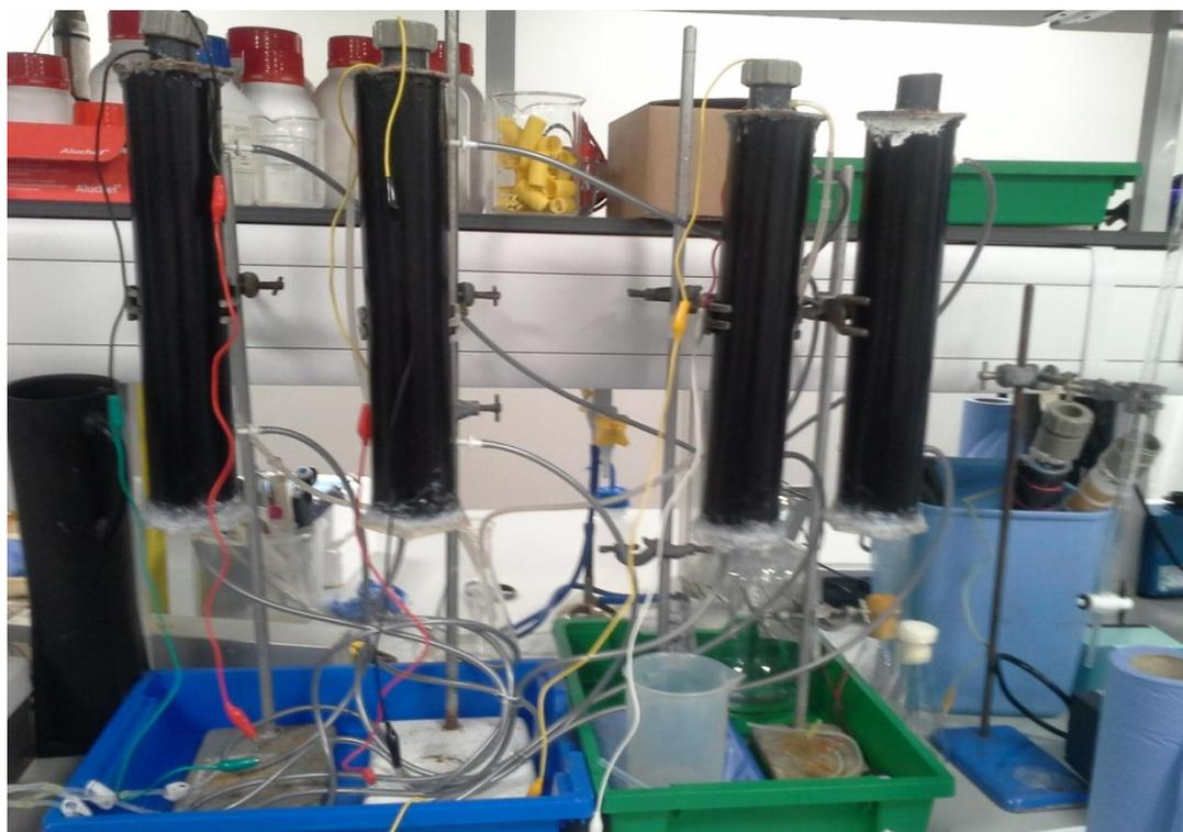
**Figure 9.2:** The experimental set-up during the start-up stage of the continuous run of the tubular MFC system for the treatment of synthetic wastewater containing petroleum hydrocarbons.
