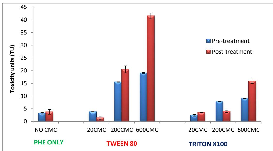
**Figure 4.9:** Toxicity response of two different surfactants at varying initial concentrations before and after treatment in a MFC using adapted microbial consortia as inoculum. The TU values are means of duplicate experiments  $\pm$  SD.
