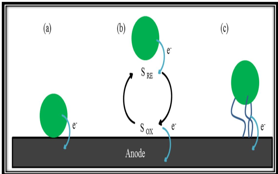
**Figure 1.15: Extracellular electron transfer mechanisms:** Microbially catalysed electron transfer from substrate reduction/oxidation onto electrode surface. This may occur either through direct contact, mobile electron shuttles or nanowires respectively, as shown above (Chouler and Lorenzo, 2015).
