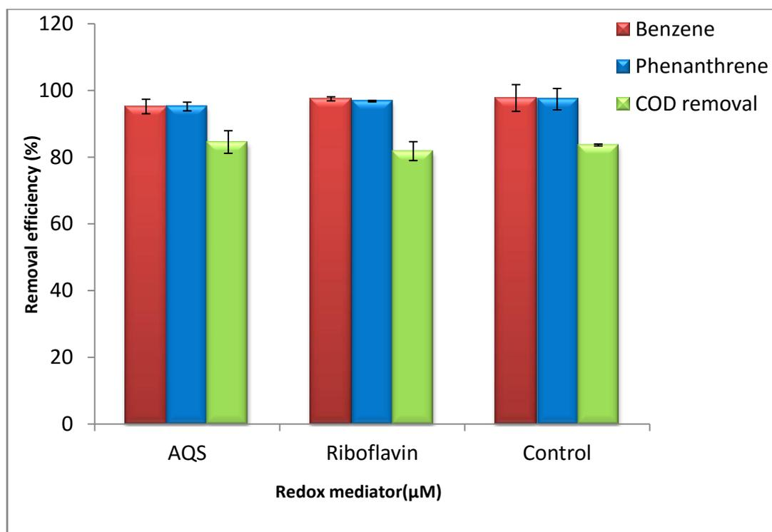
**Figure 4.5:** Effect of redox mediators on COD removal and degradation efficiencies during MFC operation using adapted anaerobic microbial consortia. Values are means of duplicate experiments  $\pm$  SD.
