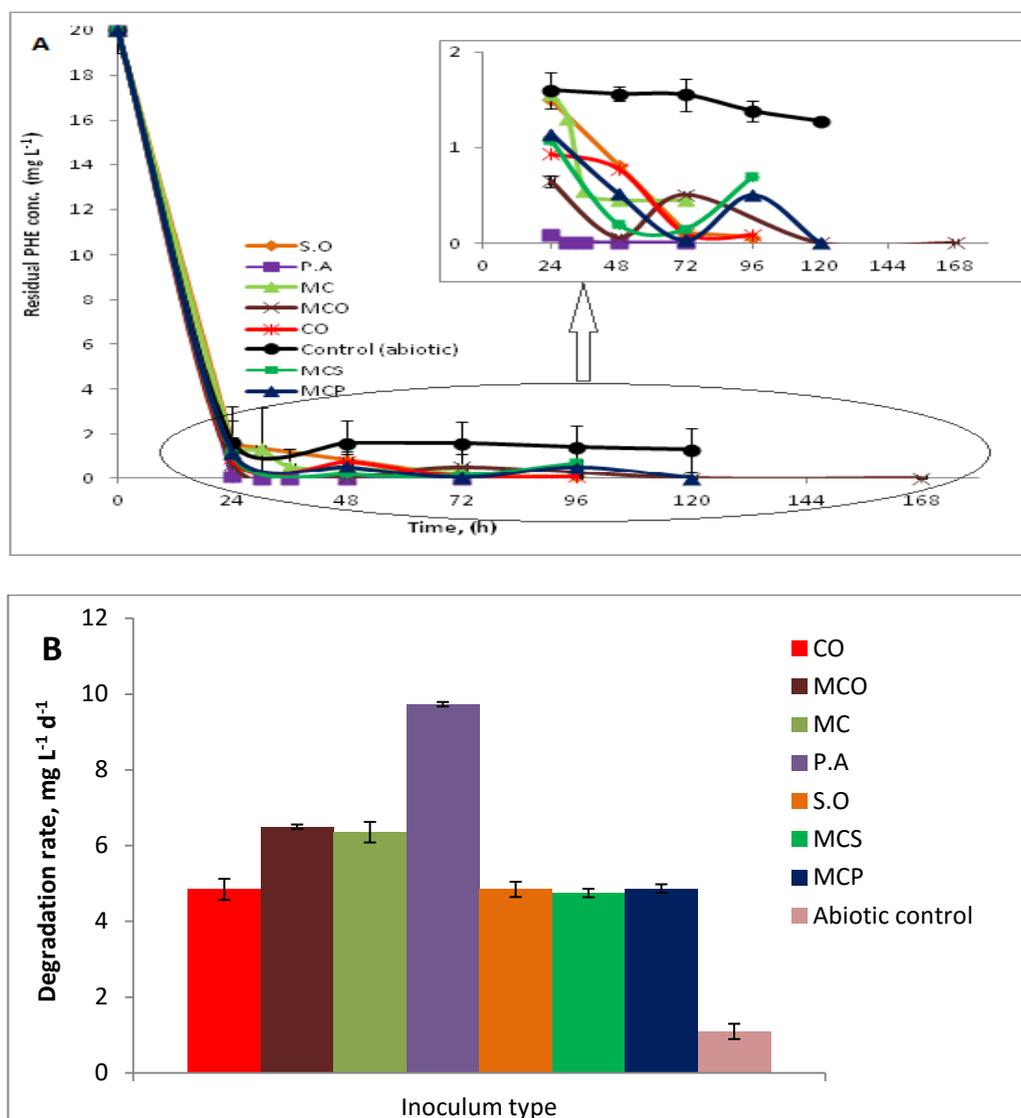
**Figure 3.2:** (A) Phenanthrene (PHE) concentration in the bulk anode solution as a function of time and inset: A clearer picture of the plot of residual phenanthrene concentration against incubation time between 24 and 170 h (B) phenanthrene (average) degradation rates by different inocula used. The error bars represent the SD of the mean
