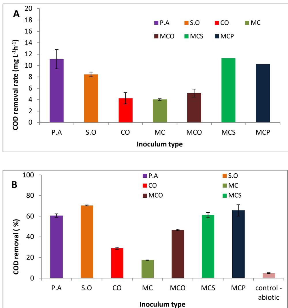
**Figure 3.6:** (A) COD % removal and (B) COD removal rate over the study period in a MFC for different strains. *S. oneidensis* (S.O), *P. aeruginosa* (P.A), a co-culture of *S. oneidensis* and *P. aeruginosa* (CO), anaerobic digested sludge (MC), anaerobic digested sludge with the co-culture (MCO), anaerobic digested sludge with *S. oneidensis* (MCS) and anaerobic digested sludge with *P. aeruginosa*, MCP. Values are means of duplicate experiments  $\pm$  SD.
