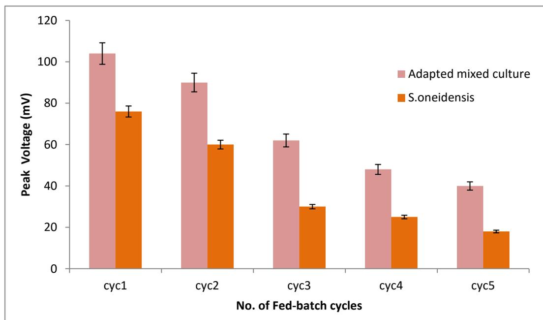
**Figure 3.11:** Comparison of peak voltages output of the two inoculum types (*S.oneidensis* MR1 and MFC-adapted mixed culture). Values are means of duplicate experiments  $\pm$  SD.
