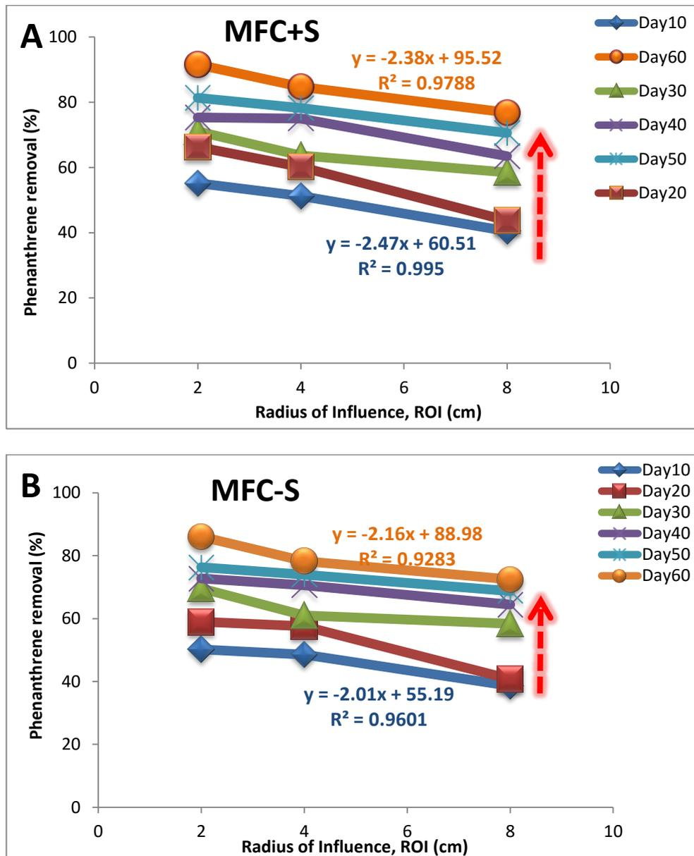
**Figure 6.2:** Relationship between phenanthrene removal and the radial distance from the MFC anodes at different sampling times. Dashed arrows indicate that maximum ROIs were expanding as reflected by the flattening of the slopes.
