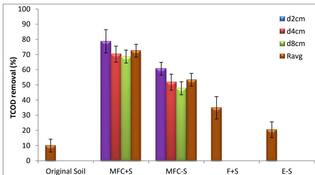
**Figure 6.4:** Percentage total COD (TCOD) removal at different distances from the anode for the active MFCs and control reactors at the end of 60 days of MFC operation at ambient temperature. Ravg is the average of removal efficiencies at different radial distance from the anode. Values are means of triplicate measurements  $\pm$  SD. E-S and F+S mean controls without and with surfactant addition respectively.
