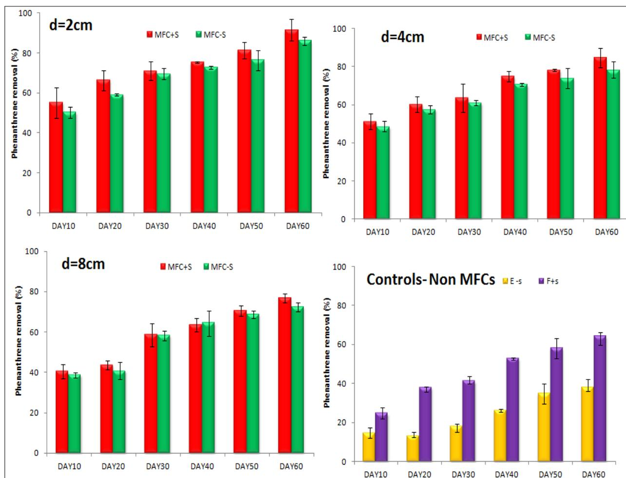
**Figure 6.1:** Phenanthrene removal in soil at distance of 2 - 8 cm from the anode during the operating period in MFCs with MFC only (MFC-S) and MFC with surfactant (Tween 80, 250 mg L<sup>-1</sup>) amendment (MFC+S) using indigenous soil microorganism as inoculum source. Controls were prepared in the same reactors but with no electrodes. Error bars  $\pm$  SD are based on triplicate measurements. E-S and F+S means controls without and with surfactant addition respectively.
