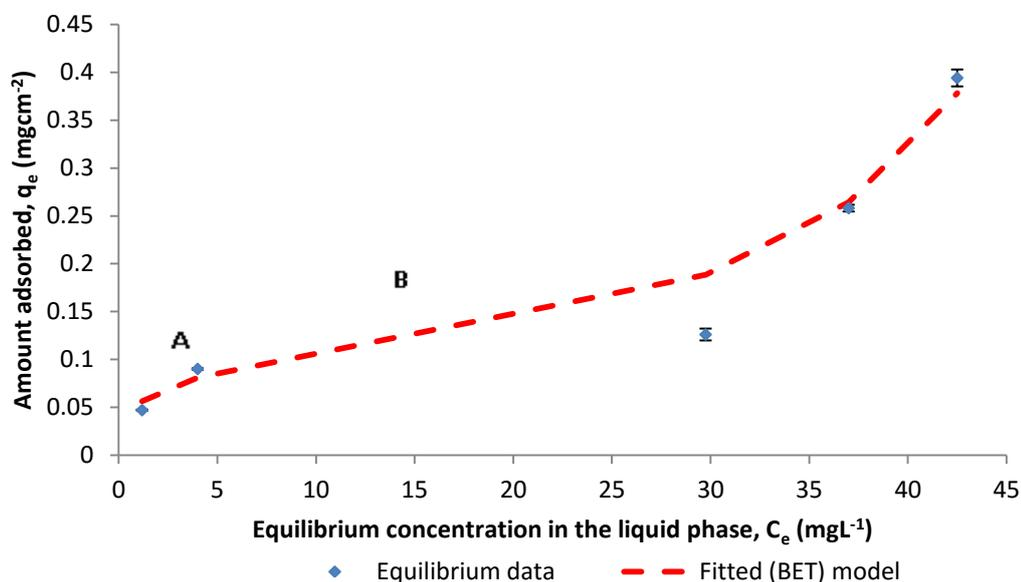
**Figure 3.1:** Adsorption isotherm of phenanthrene onto carbon felt [pH = 7; contact time = 180 mins; agitation speed: 0 rpm; adsorbent's surface area =  $40 \text{ cm}^2$ , T =  $30^\circ\text{C}$ ]. The error bars represent the SD of the mean.
