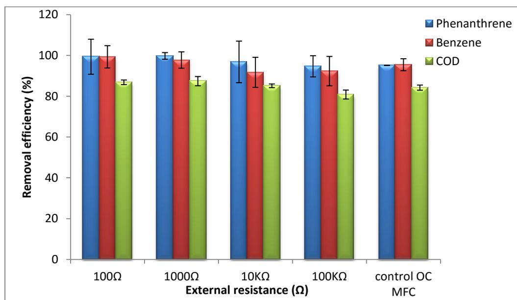
**Figure 4.10:** Degradation and COD reduction performance of MFC systems at various external resistances compared to open circuit control during 10 days of operation using adapted mixed culture at incubation temperature of  $30 \pm 3^\circ\text{C}$ . Values are means of duplicate experiments  $\pm$  SD.
