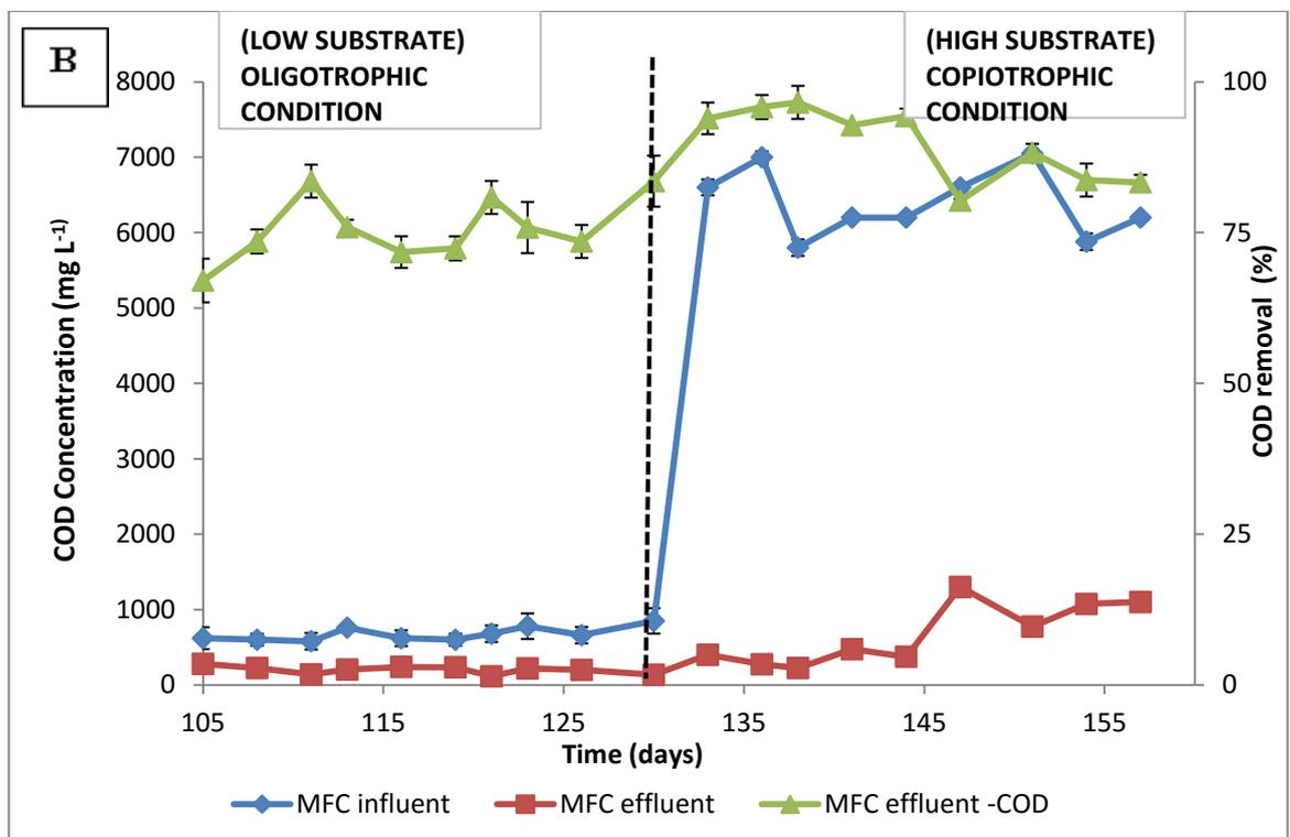
**Figure 5.5:** (A) Degradation performance of the tubular MFC at high substrate condition (B) COD removal at low and high substrate conditions operated in a continuous mode at HRT of 10 d. Error bars  $\pm$  SD are based on duplicate measurements.
