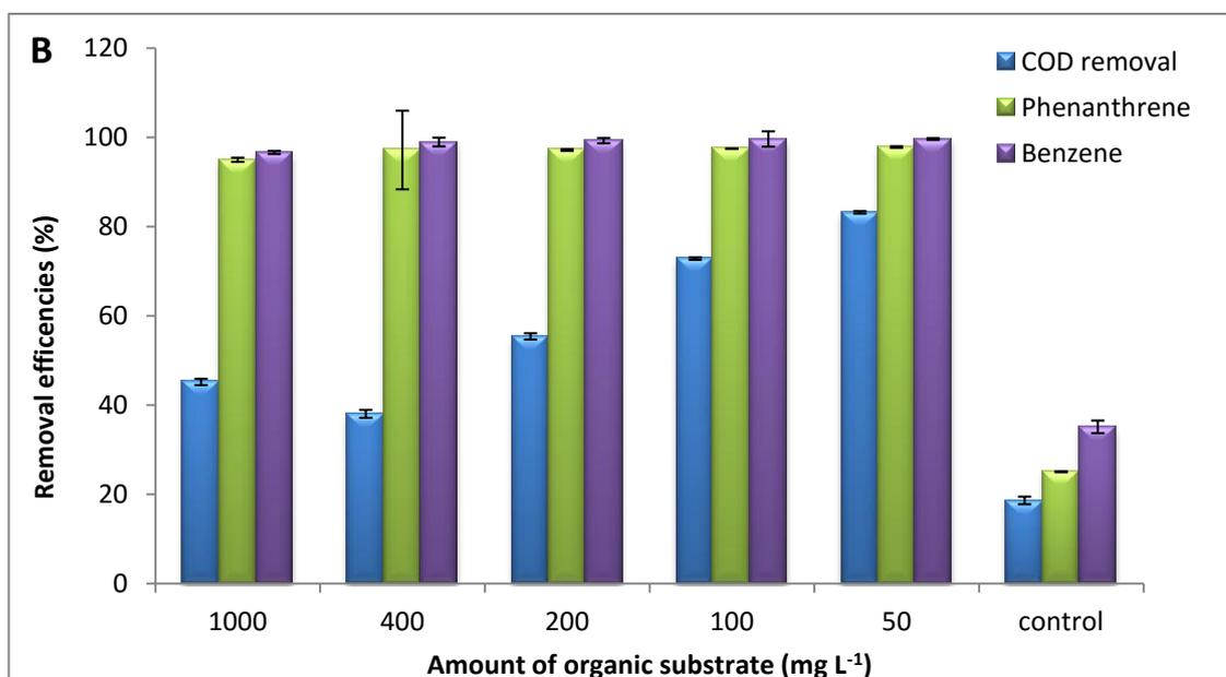
**Figure 3.12:** Removal efficiencies for degradation of phenanthrene and benzene using (A) *S. oneidensis* MR1 and (B) MFC-adapted mixed culture as inoculum respectively. Values are means of duplicate experiments  $\pm$  SD.
