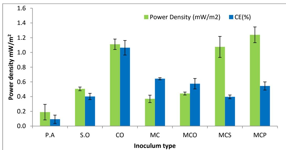
**Figure 3.5:** Comparison of power densities outputs and coulombic efficiencies for different inoculum types. Coulombic efficiency (CE), *S. oneidensis* (S.O), *P. aeruginosa* (P.A), a co-culture of *S. oneidensis* and *P. aeruginosa* (CO), anaerobic digested sludge (MC), anaerobic digested sludge with the co-culture (MCO), anaerobic digested sludge with *S. oneidensis* (MCS) and anaerobic digested sludge with *P. aeruginosa*, MCP. Values are means of duplicate experiments  $\pm$  SD.
