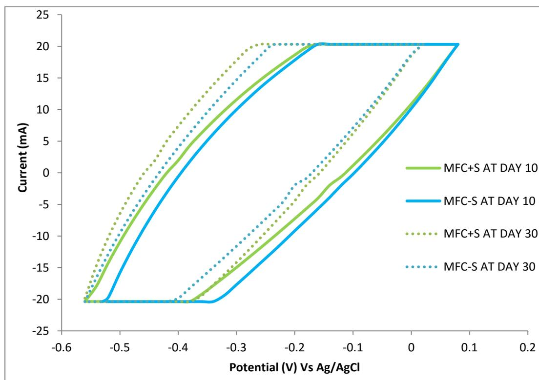
**Figure 6.7:** The CV curve for phenanthrene in MFC only (MFC-S) and MFC with surfactant (Tween 80,  $250 \text{ mg L}^{-1}$ ) amendment (MFC+S) at day 10 (solid line) and day 30 (dashed line) at sweep rate of  $10 \text{ mVs}^{-1}$ .
