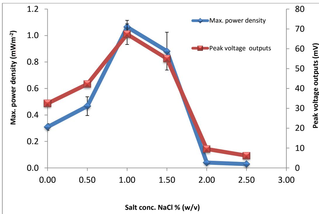
**Figure 4.2:** The effect of salinity on electrochemical performance of the MFC system at temp. 30°C using adapted anaerobic microbial consortia.. Values are means of duplicate experiments  $\pm$  SD.
