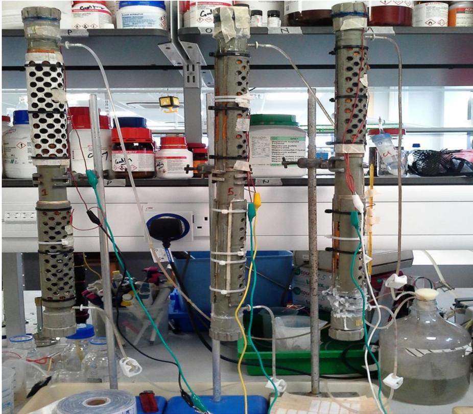
**Figure 9.4:** The MFC system (during start-up of the continuous run) used for the treatment of petroleum hydrocarbon containing synthetic wastewater.
