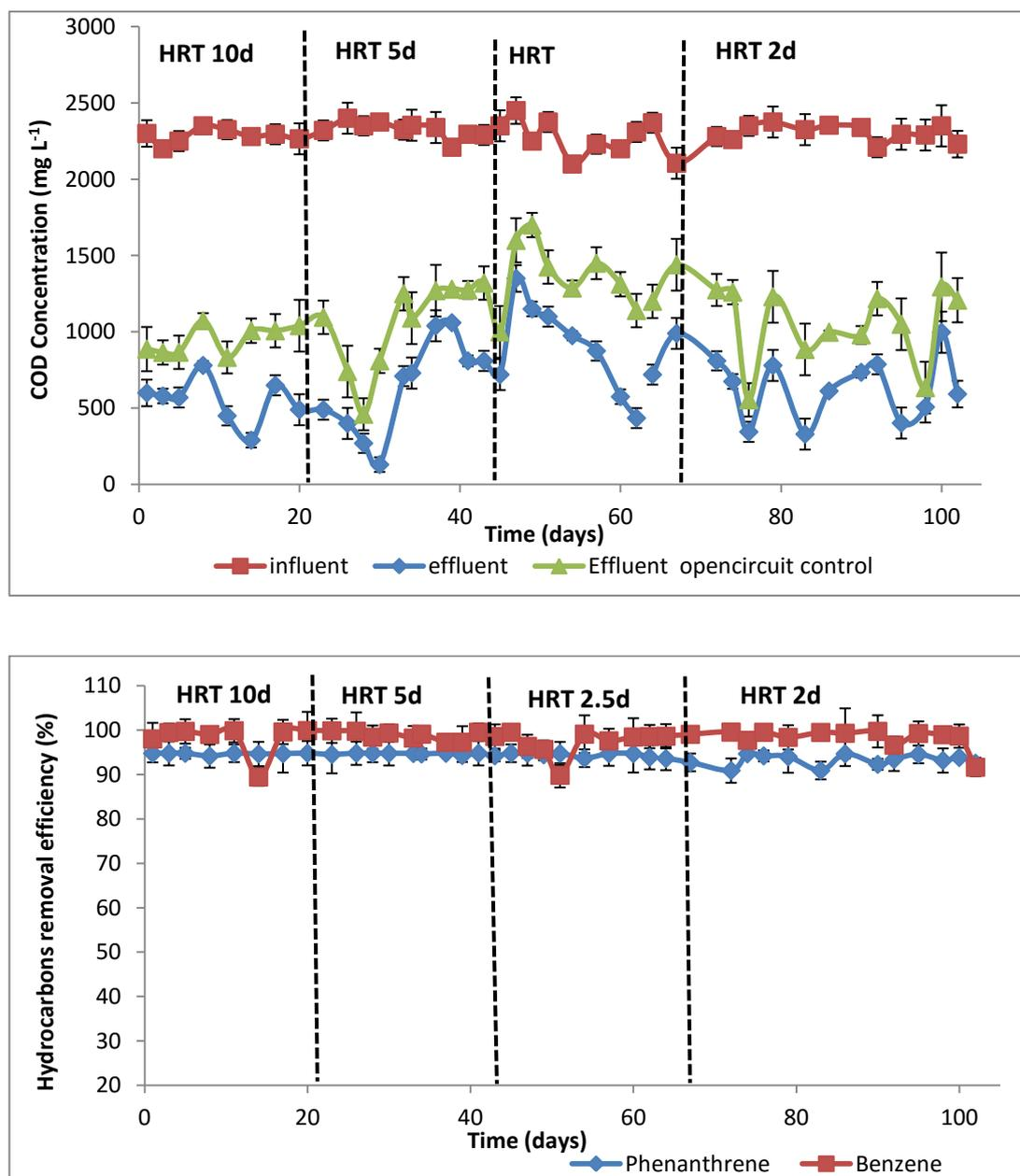
**Figure 5.1:** (A) COD removal and (B) Hydrocarbons removal efficiencies at various HRT regimes over a period of 110 days of continuous MFC operation at ambient temperatures (14-25 °C) using adapted microbial consortia. Values are means of duplicate experiments  $\pm$  SD.
