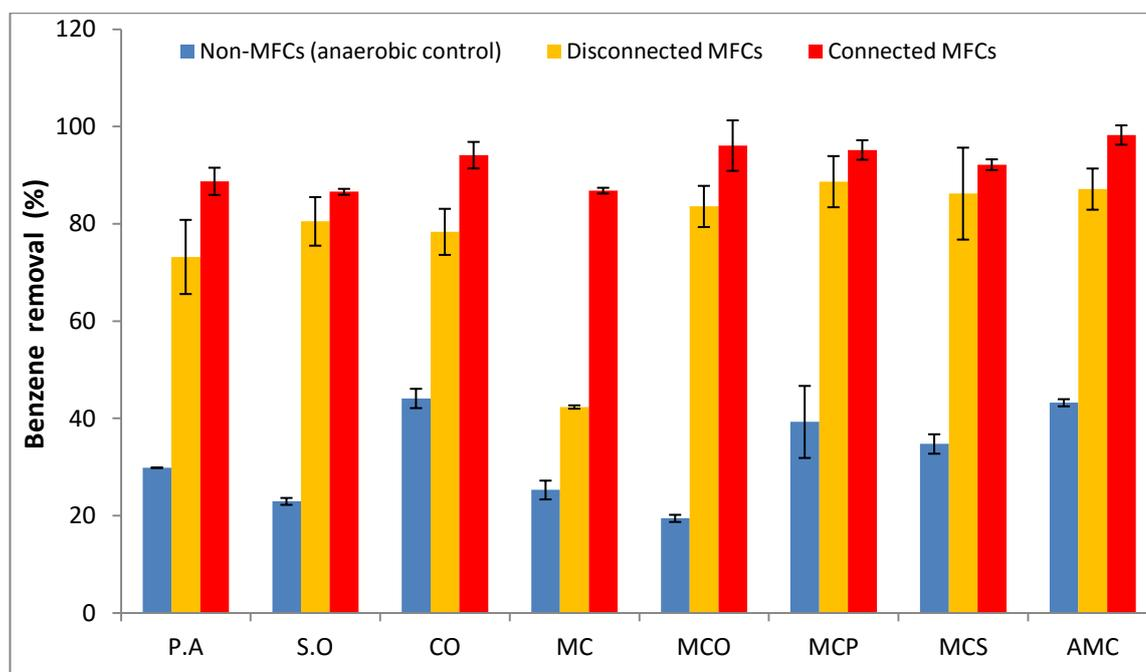
**Figure 3.8:** Degradation efficiencies for benzene removal by different inoculum types. *S. oneidensis* (S.O), *P. aeruginosa* (P.A), a co-culture of *S. oneidensis* and *P. aeruginosa* (CO), anaerobic digested sludge (MC), anaerobic digested sludge with the co-culture (MCO), anaerobic digested sludge with *S. oneidensis* (MCS), anaerobic digested sludge with *P. aeruginosa*, MCP and adapted mixed culture (AMC). The error bars represent the SD of the mean.
