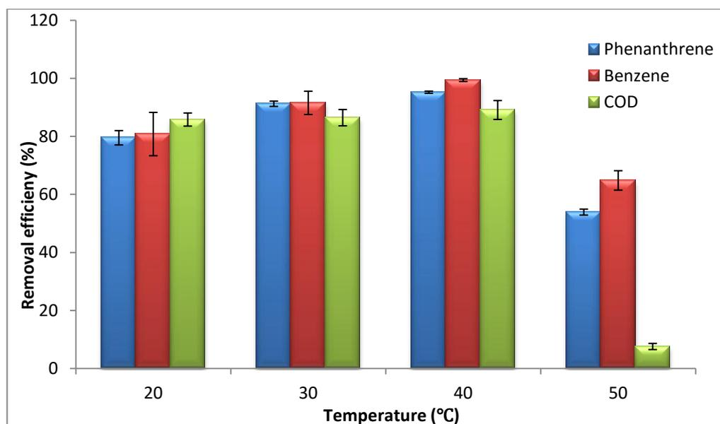
**Figure 4.4:** Effect of operating temperature on COD removal and degradation efficiencies during MFC operation using adapted anaerobic microbial consortia. Values are means of duplicate experiments  $\pm$  SD.
