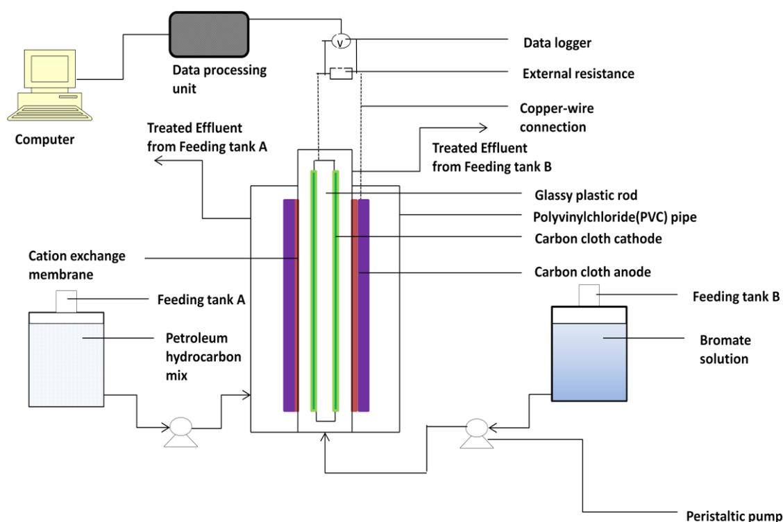
**Figure 2.2:** A schematic diagram of the tubular MFC reactor in an up-flow configuration for the treatment of hydrocarbon-containing synthetic wastewater for *in situ* applications.
